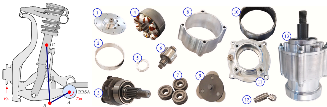
Figure 9: The Rotary Regenerative Shock Absorber (RRSA) design by [8] showing linkage positioning on a McPherson strut geometry and individual components, including two stage planetary gearbox and generator rotor and stator.
